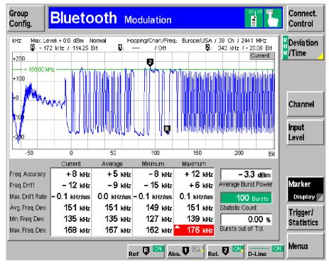
Fig. 2 Bluetooth Modulation Display
